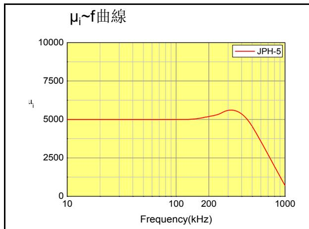
Test core: OD=25mm TH=8mm ID=15mm
